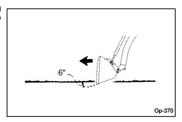
With bucket level, start a cut at notch approximately 2 inches deep. Hold depth by feathering bucket control to adjust cutting lip up or down. When front tires enter the notch, adjust lift cylinder to maintain proper depth.
